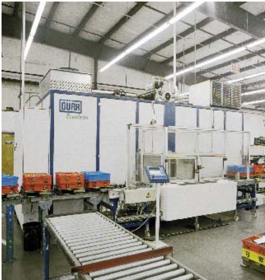
Watts Regulator Company has been using the Universal 71C dual-chamber hydrocarbon system since October 2000.
