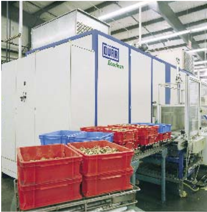
Target volume for cleaning on the Dürr Ecoclean is 60 baskets per hour.
