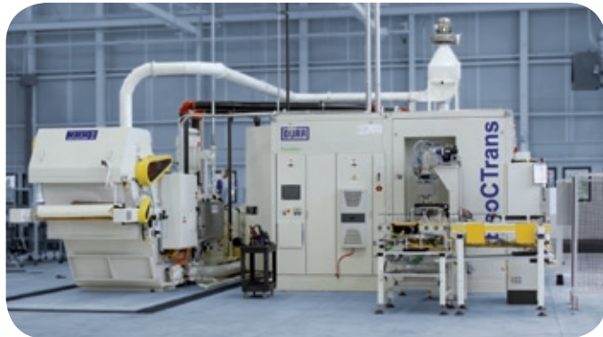
Dürr Ecoclean's EcoCTrans cleaning machine (right) with external TRVD vacuum filter (left).
