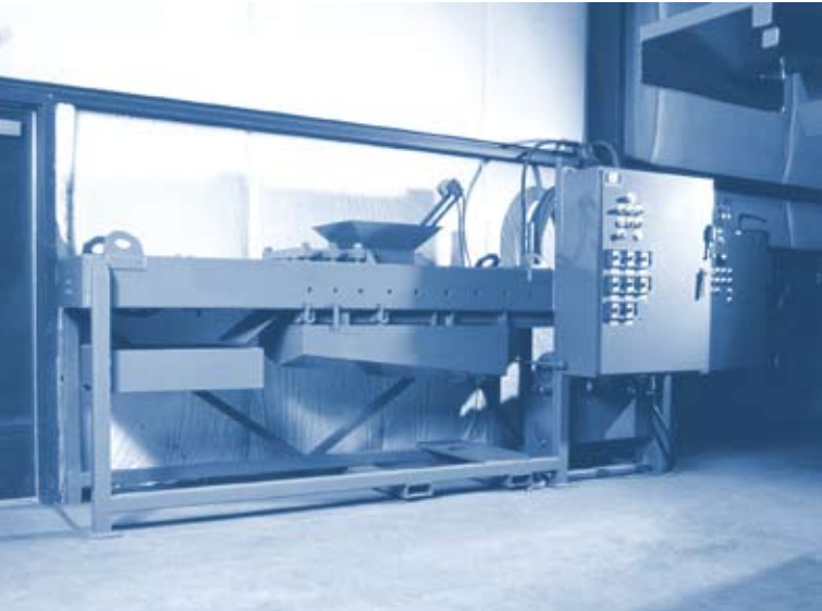
Briquetter operates automatically, prompted either by a full load, or by the start of a timed index cycle
