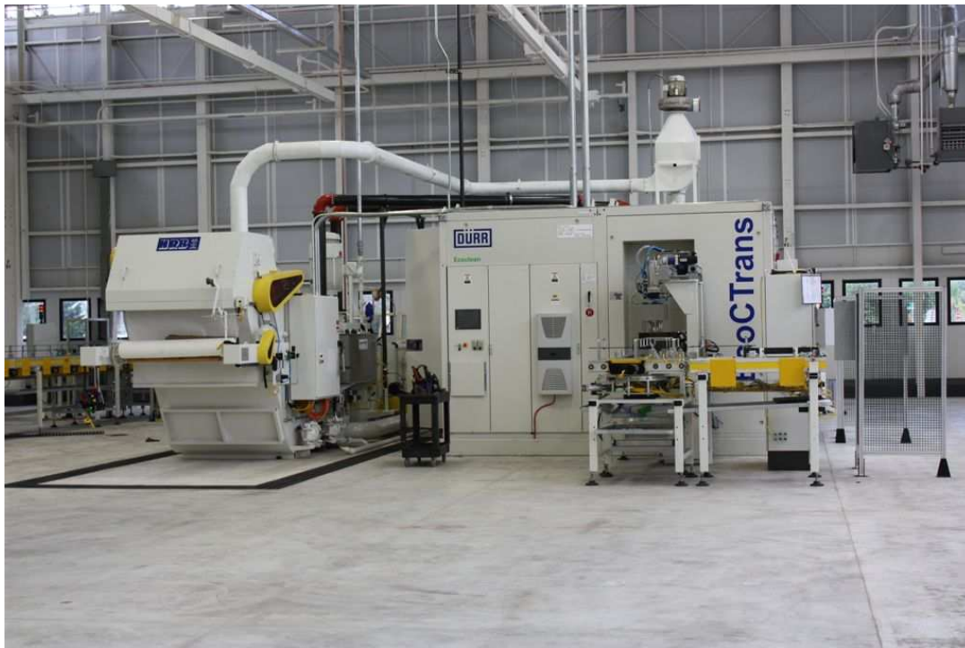
Ecoclean equipment on site: an EcoCTrans washer and an HRB filter
